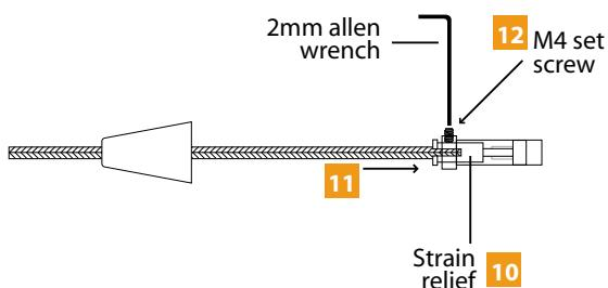
**10** The strain relief slots should be rotated 90° away from the M4 set screw.
