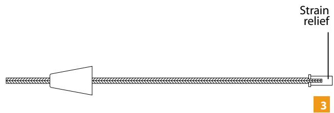
**3** Insert the coaxial cable through the flared end of the strain relief.
