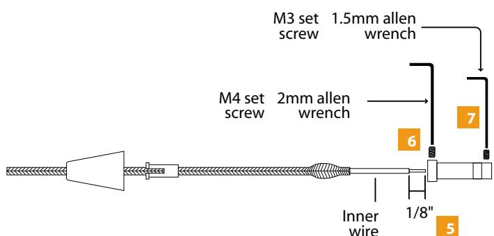
**5** Strip 1/8" from end of the inner wire. Make sure that the stripped portion is not greater than 3/16".
