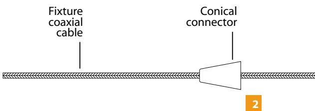
**2** Insert the fixture coaxial cable through the conical connector
