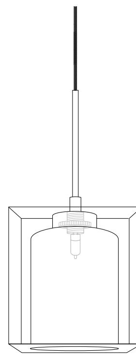
**1** Feed coaxial cable as shown through applicable glass.
