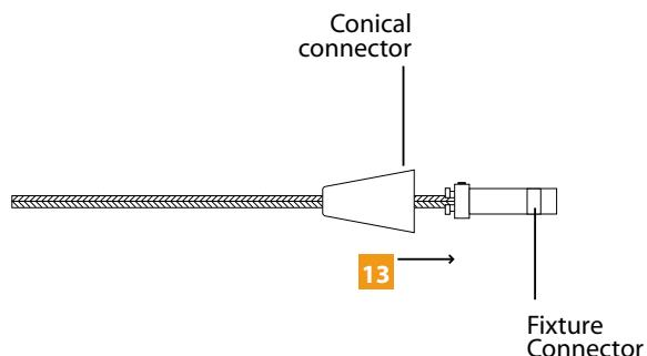
**8** While inserting the inner wire into the connector look through the set screw hole to make sure that the stripped portion of the inner wire contacts end of the connector.
