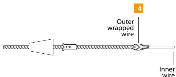
**4** Slide the outer wrapped wire back to expose the inner wire.
